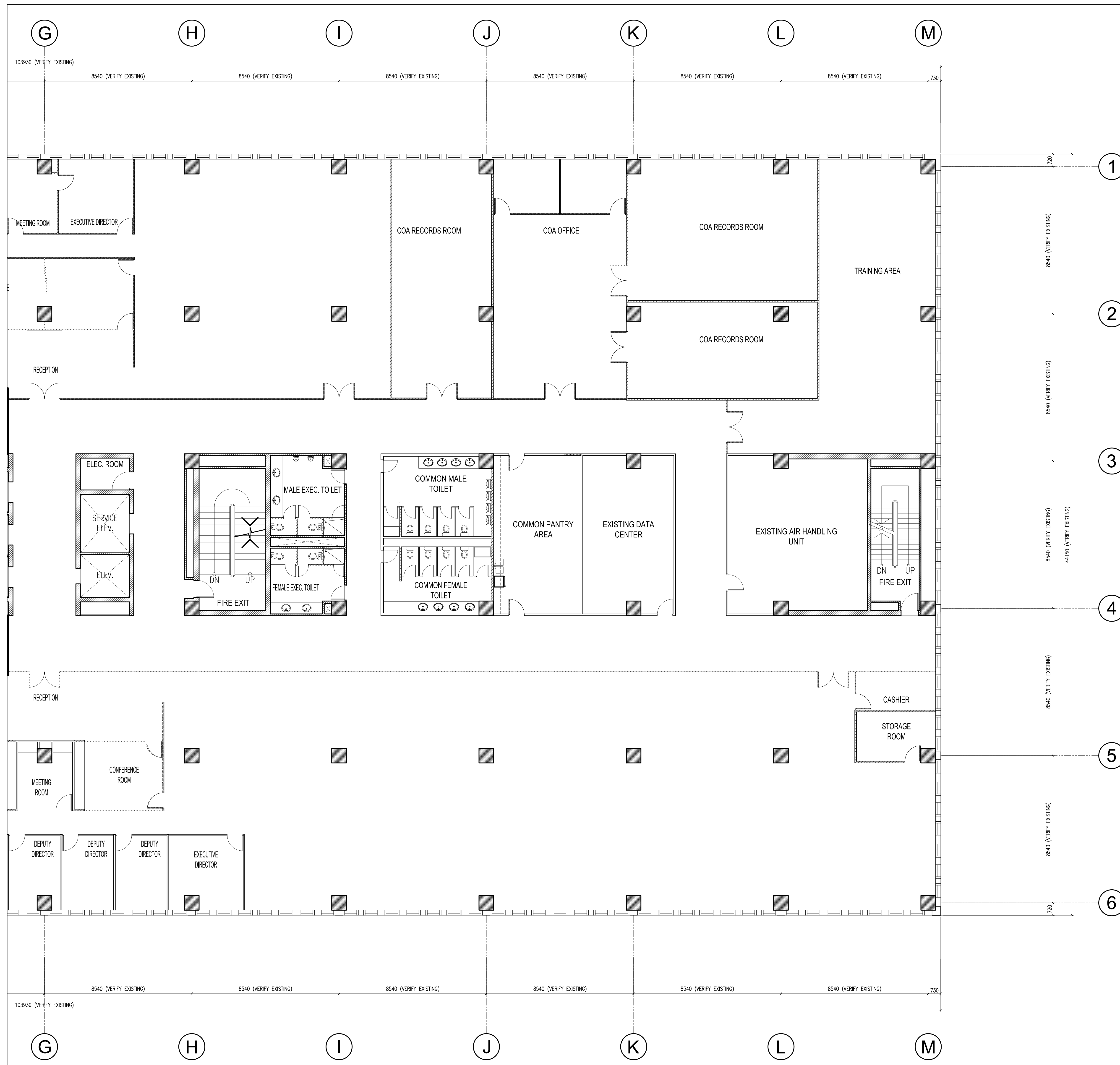
DEPARTMENT OF FINANCE 8TH FLOOR EDCP BUILDING RENOVATION PROJECT (NTRC AND FIRB OFFICES) 1 AS-FOUND WALL PLAN AND PROPOSED DEMOLITION & DISMANTLING PLAN B SCALE: A-2.2 1:100 MTS
