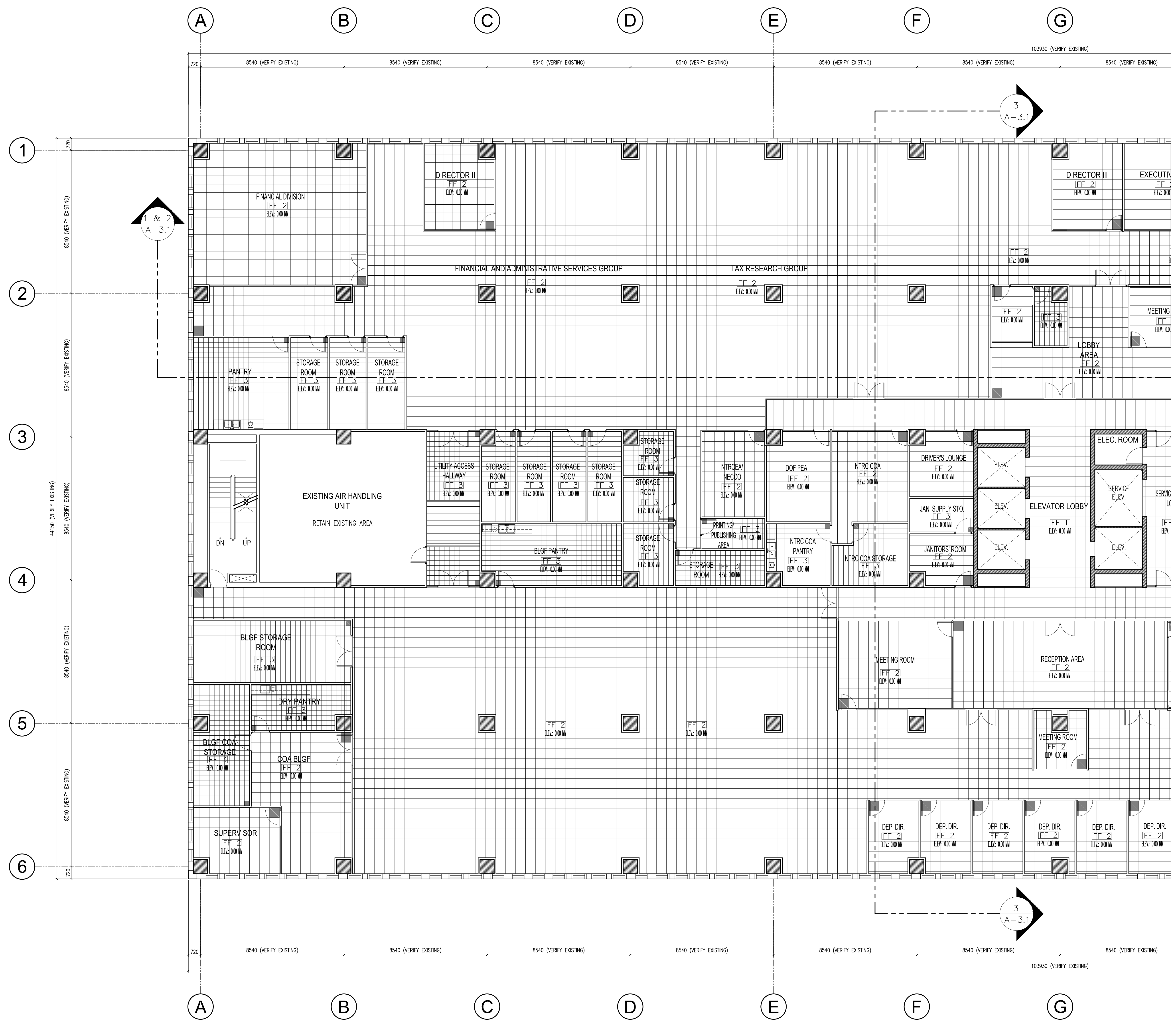
UPDATED SCHEME 7A (NTRC AND FIRB OFFICES) DEPARTMENT OF FINANCE 8TH FLOOR EDCP BUILDING 1 FLOOR FINISH LAYOUT A A-2.7 SCALE NTS
